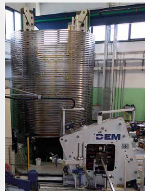
Compaction of 50x50 mm square tube used to implement nuclear fusion plant (ITER).
